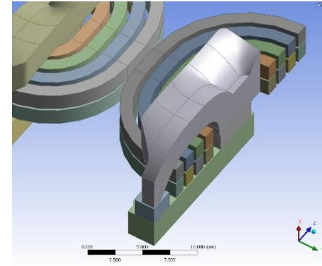
IBM developed a **new high moment (HM) layered pole write head** that produces much larger magnetic fields enabling the use of smaller magnetic particles
